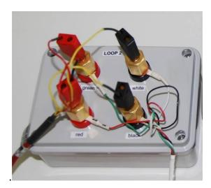
The connection unit is connected to the front connection of 34420A. Measured values can be read on display or via GIPB interface bus. When thermometer is connected and 34420A switched on, the temperature of the thermometer can be observed by pressing SHIFT and TEMP key. The display shows temperature of Pt100 in degrees Celsius.
