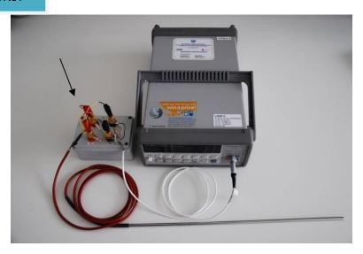
The thermometer is connected (4 wire) to the connection unit as follows:
