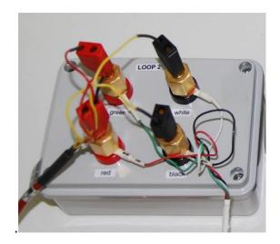
The connection unit is connected to the front connection of 34420A. Measured values can be read on display or via GIPB interface bus. When thermometer is connected and 34420A switched on, the temperature of the thermometer can be observed by pressing SHIFT and TEMP key. The display shows temperature of Pt100 in degrees Celsius.
