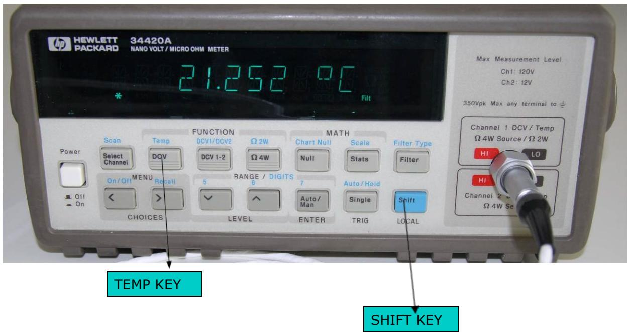
If thermometers reading via GPIB is preferred, following setup for 34420A is used:
